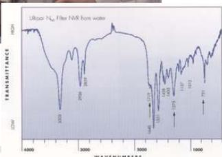
FTIR spectroscopy is used for identification of extractable materials.
