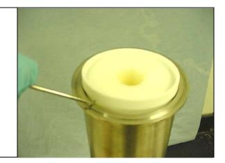
• Using the o-ring pick, remove the outer o-ring. Insert the pointed end of the pick into the o-ring and pull outward.
