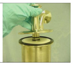
• Install the clamps using a 3/8" socket.
