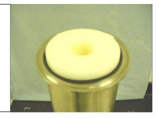
• Place the large insertion tool over the end of the cartridge and outer oring. Tap lightly on the insertion tool until the cartridge is <u>centered</u> in the housing.
