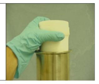
• Position an outer o-ring over the potted end. Note that the cartridge will be about 1/4" below the flanged surface of the housing.
