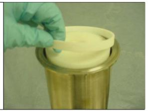
• Install a gasket in the grooved end of the housing.
