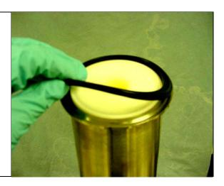
• Using the o-ring pick, remove the retention ring.
