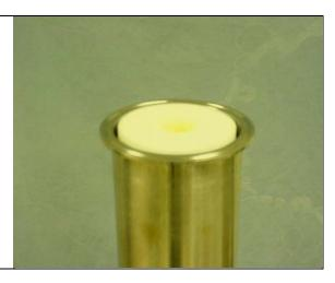
• Install a retention ring on one side of the contactor. Tap lightly with the rubber mallet if necessary.
