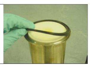
NOTE: Prior to inserting the end cap, check the integrity of the 2 small center o-rings. Replace if damaged or worn.
