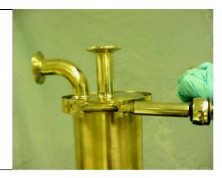
• Remove the end caps using a twisting, pulling motion. It may be necessary to lightly tap the gas elbow outward with a rubber mallet to loosen the end cap.
